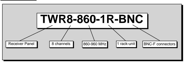
Receiver Distribution Panels Ship Standard With N-Female Connectors Standard Power Supply Voltages Available:
